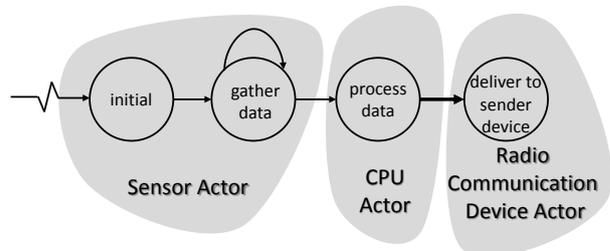
Fig. 3. How events of a WSN sensor are associated with actors
