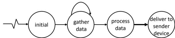
Fig. 2. The event graph of a WSN sensor behavior
