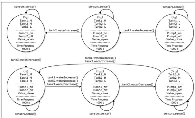
Figure 6: The abstracted state transition of SWaT system.
